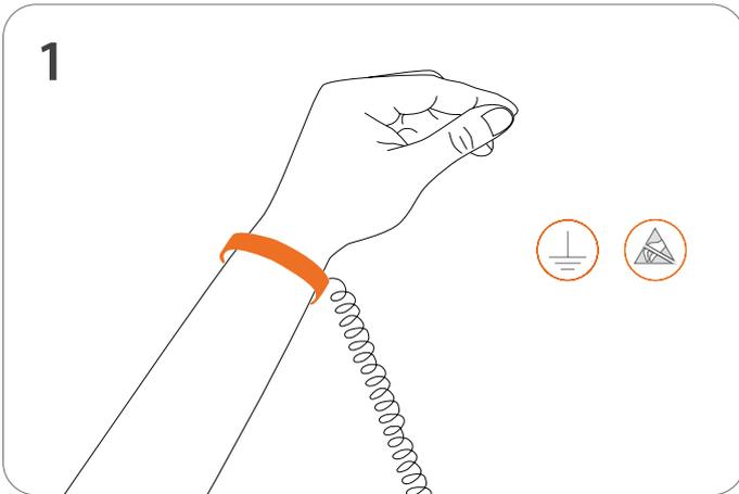
1 Work in an ESD protected environment. Make use of an anti-static strap.
