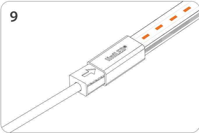
Test the liniLED® LED strip before you slide it fully over the clamp (4).
