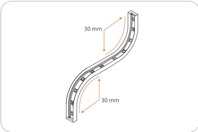
Maximum bending radius is 30 mm. Solely bend up or downward.
