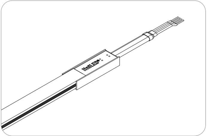
Submersible, chlorine resistant | (IP68) | Welded Connector
