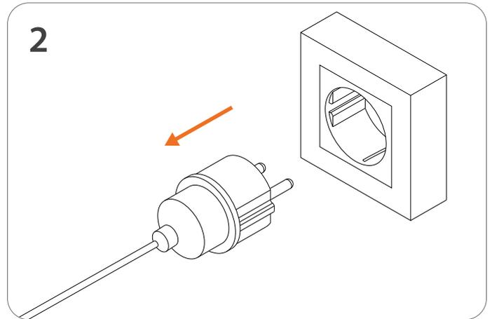
2 Turn off the power before cutting the LED strip.
