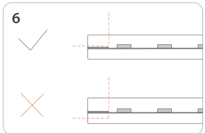
6 Isometric view | Do **not** cut the PCB!
