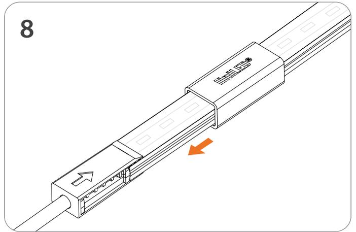
Slide the shell (2) partly over the clamp (4).
