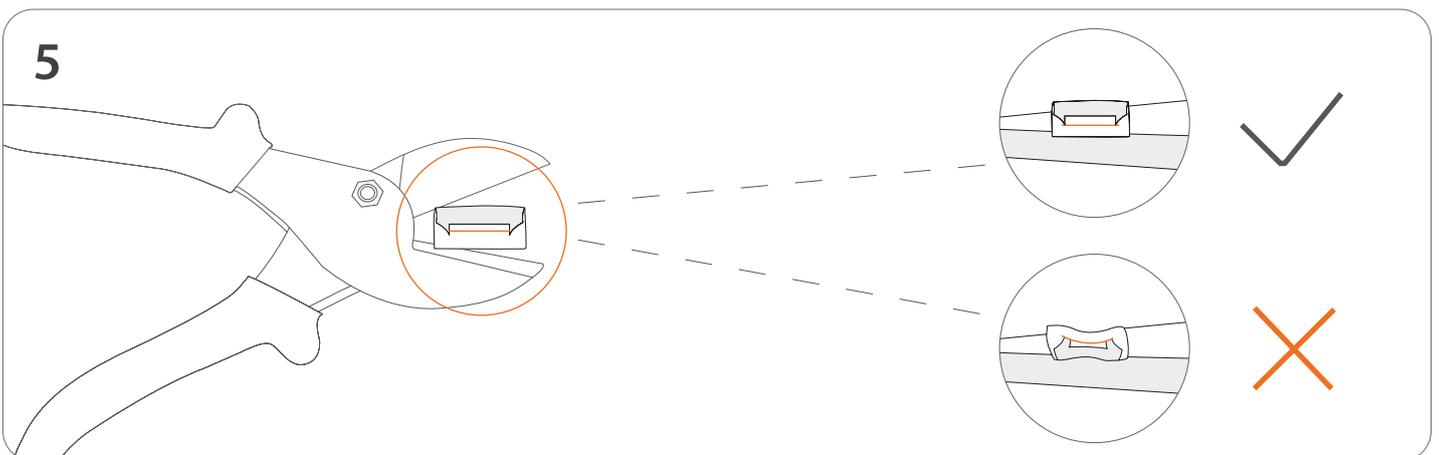
5 Top view | Only cut on the dotted lines to prevent damaging the LED strip.
