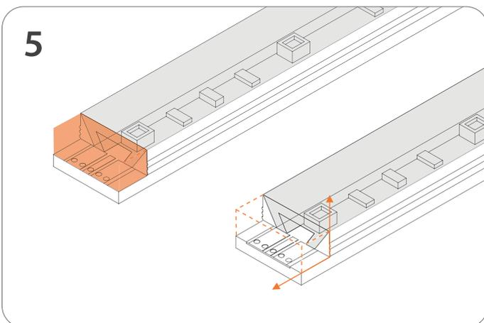
5 Isometric view | Only cut the LED strip extrusion on the dotted line of the extrusion to prevent damaging the PCB. Carefully cut away this part of the extrusion.
