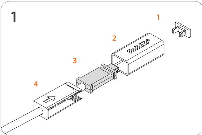
The liniLED® IP40 Connector consists of: End cap (1), Shell (2), Connector (3), Clamp (4). mm<sup>2</sup>
