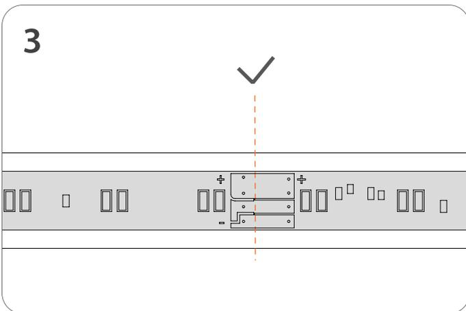
3 Top view | Make sure the cut is vertical as illustrated in the image above.
