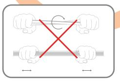
▲ Do **not** twist, stretch or compress the liniLED® LED strips.
